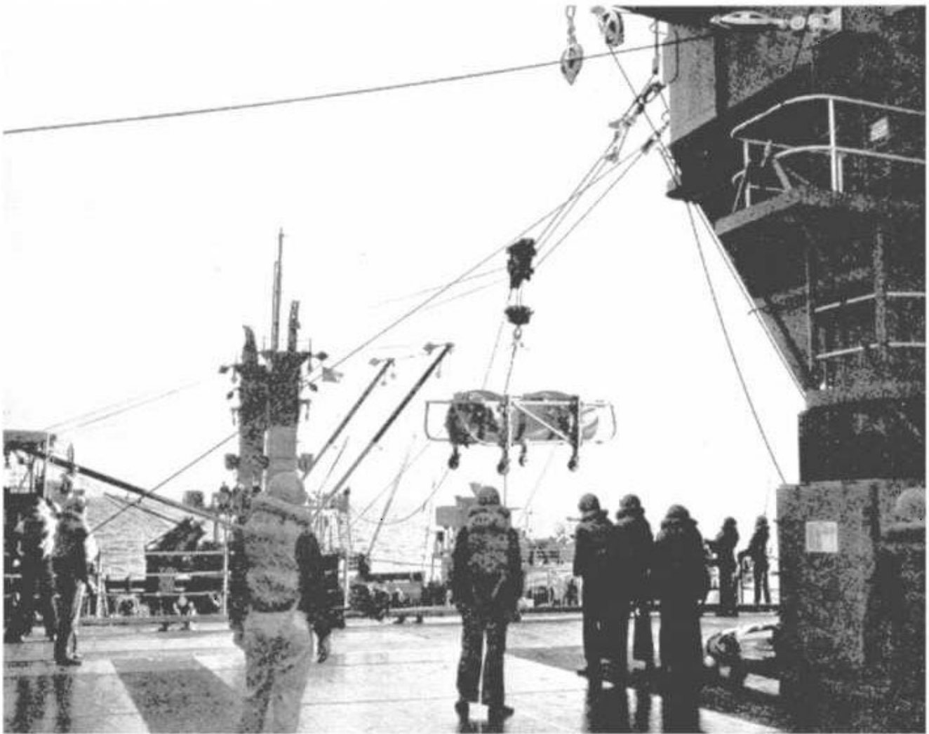
Figure 8-34.—An AE highlines a missile to a guided-missile ship during replenishment at sea.
