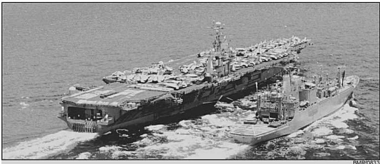
Figure 8-33.—USS John C. Stennis (CVN 74) off-loads ammunition onto ammunition ship USS Mount Hood (AE 29).
