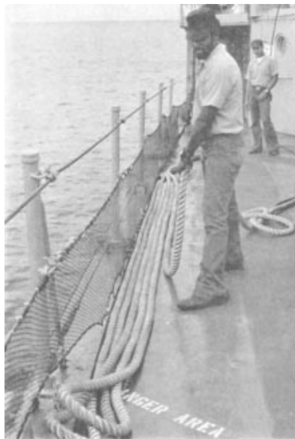
Figure 3-4.—Faking down a line. 80.22
