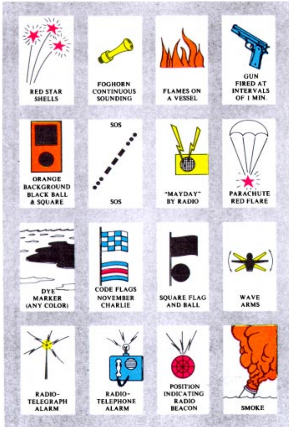
Figure 5-17.--International/inland distress signals.
