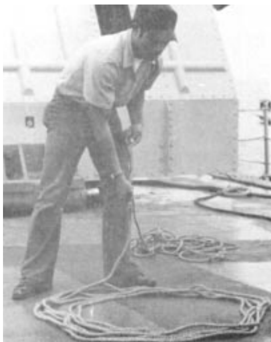
Figure 3-3.—Coiling down a line. 80.21
