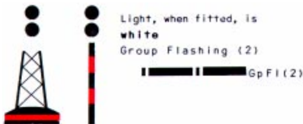
Figure 5-30.—IALA Maritime Buoyage System isolated danger marks.
