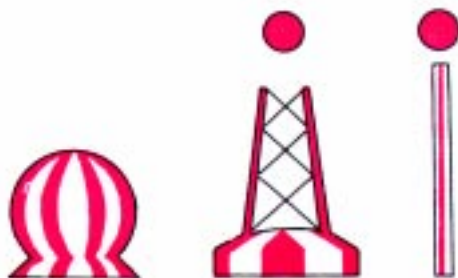
Figure 5-31.—IALA Maritime Buoyage System safe water marks.
